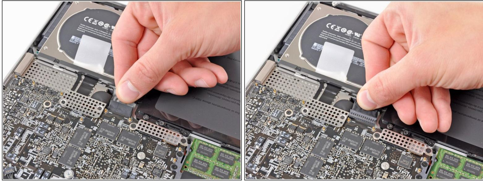
**⚠** Whenever working near the logic board, it is always wise to first disconnect the battery to avoid short circuits.
